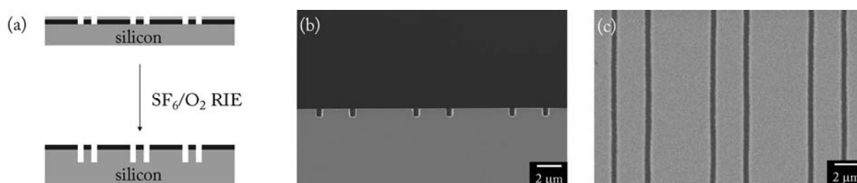
Figure 4.5 (a) Schematic representation of the RIE process. (b) High-resolution cross-sectional SEM image of 500 nm-wide trenches after etching 650 nm into silicon using SF 6 /O 2 RIE (APC open, 50 W RF power, 40 sccm SF 6 , and 20 sccm O 2 , 90 s). A clear undercut on the order of 100 nm was found, resulting in a widening of the silicon trenches with respect to the lateral dimensions in the gold mask (350 nm). (c) Low-resolution SEM image of the same structures in top view.
